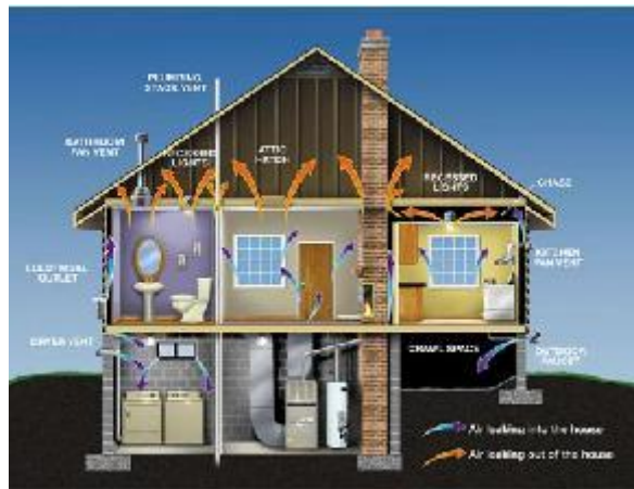
Common Air Leaks From http://www.energystar.gov/
